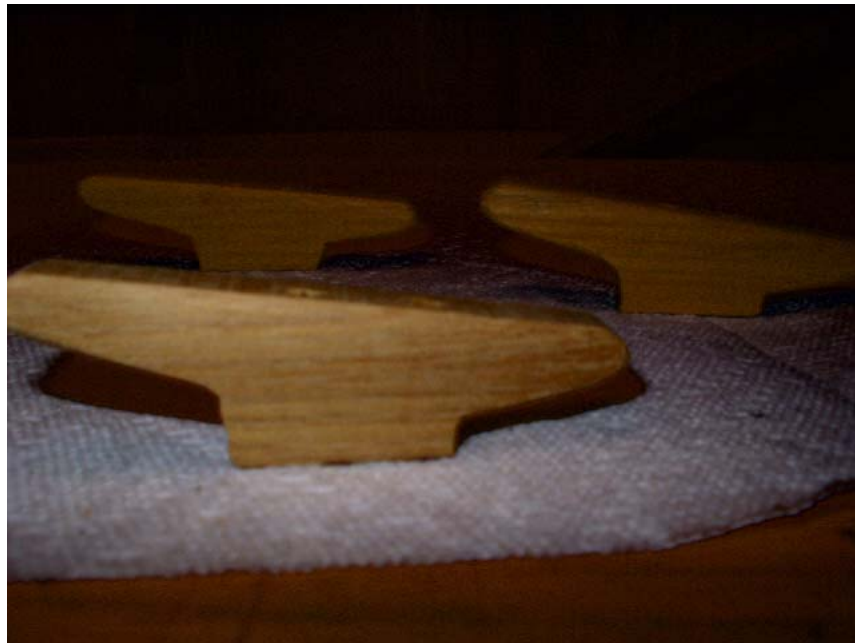
Sanded and drilled for #6 screws: a 5/32 clearance hole from the top through the base. Ready for oil finish.
