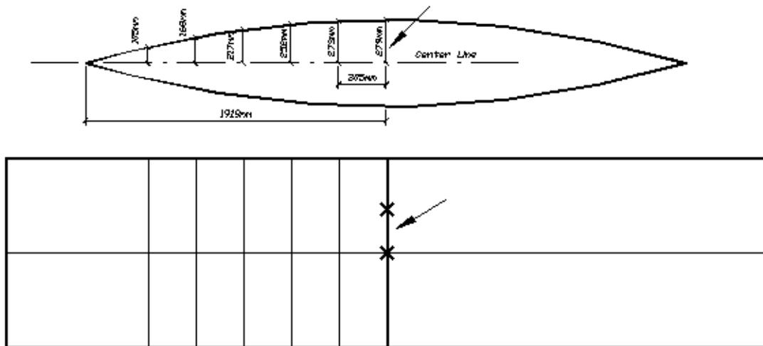
The second point is on the first line (at 305 mm from the edge) and the distance above the centerline is 273 mm. Mark it.
