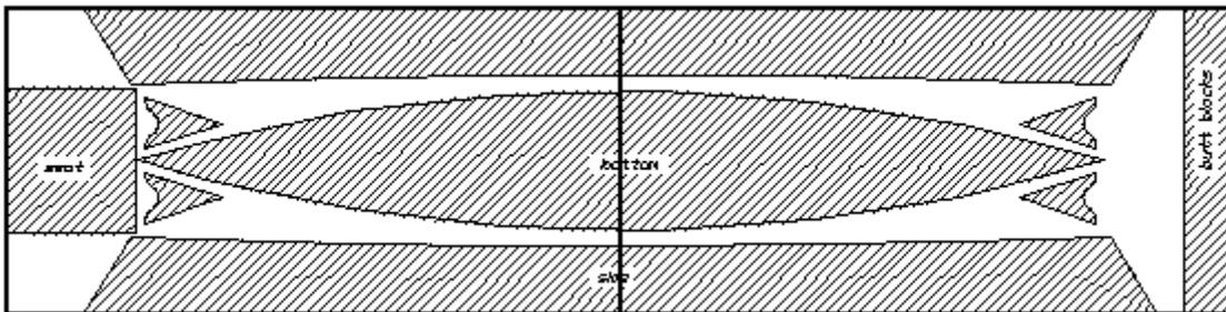
Also look at the drawing with the dimensions: everything will be measured from a centerline drawn lengthwise in the middle of those panels and from the edge between the plywood sheets. Those two lines from which we measure are called a coordinate system. All measurements must be taken from those straight lines.
