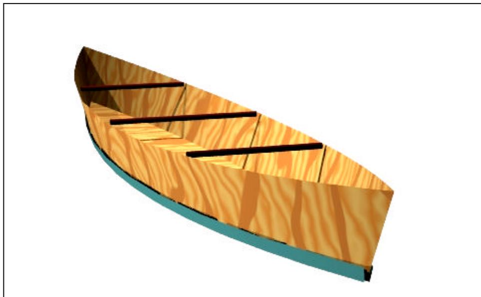
This ends the assembly phase. The next step is the fiberglass work.
