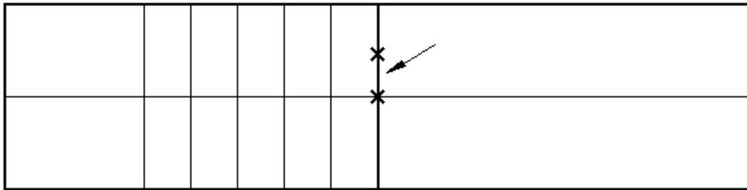
The second point is on the first line (at 305 mm from the edge) and the distance above the centerline is 273 mm. Mark it.
