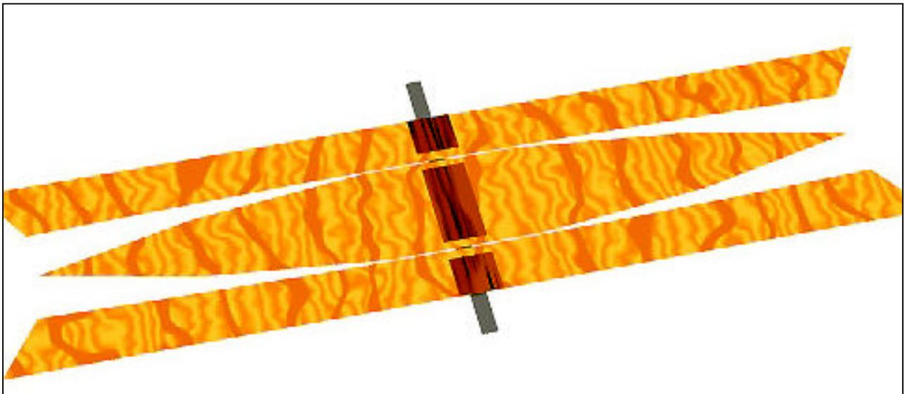
There should be piece of duct tape under the panels, full width. The tape will act as a hinge.
