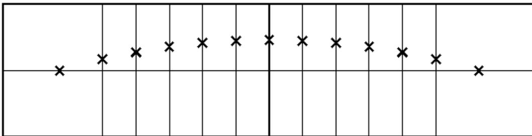
All the points for one side of the bottom panel are now on the plywood and all that is left to do is to scribe a nice smooth curve passing through all those points.
