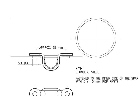
HOLE IN THE SPAR FITTED INTO THE EYE SIZE
