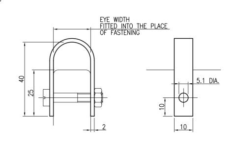
EDGE EYE STAINLESS STEEL FASTENED WITH AN M5 STAINLESS STEEL BOLT
